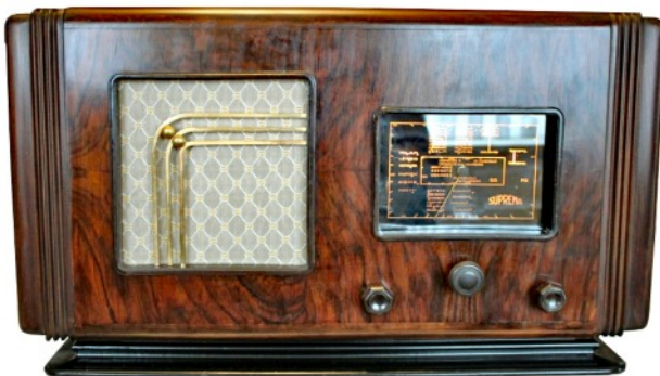
The Belgian 'Suprema' model 6A broadcast receiver was manufactured in 1937/38. It covered medium and long wave and was powered from AC mains. The receiver was built by Suprema, believed to be located in Antwerp, using the chassis of an SBR 374A. It comprised a superheterodyne circuit with an RF stage, mixer, IF stage (123kHz), which was also used as an AF stage in reflex, and an AF output stage. The valves used were 6D6, 6A7, 6B7, 42, and 80.
