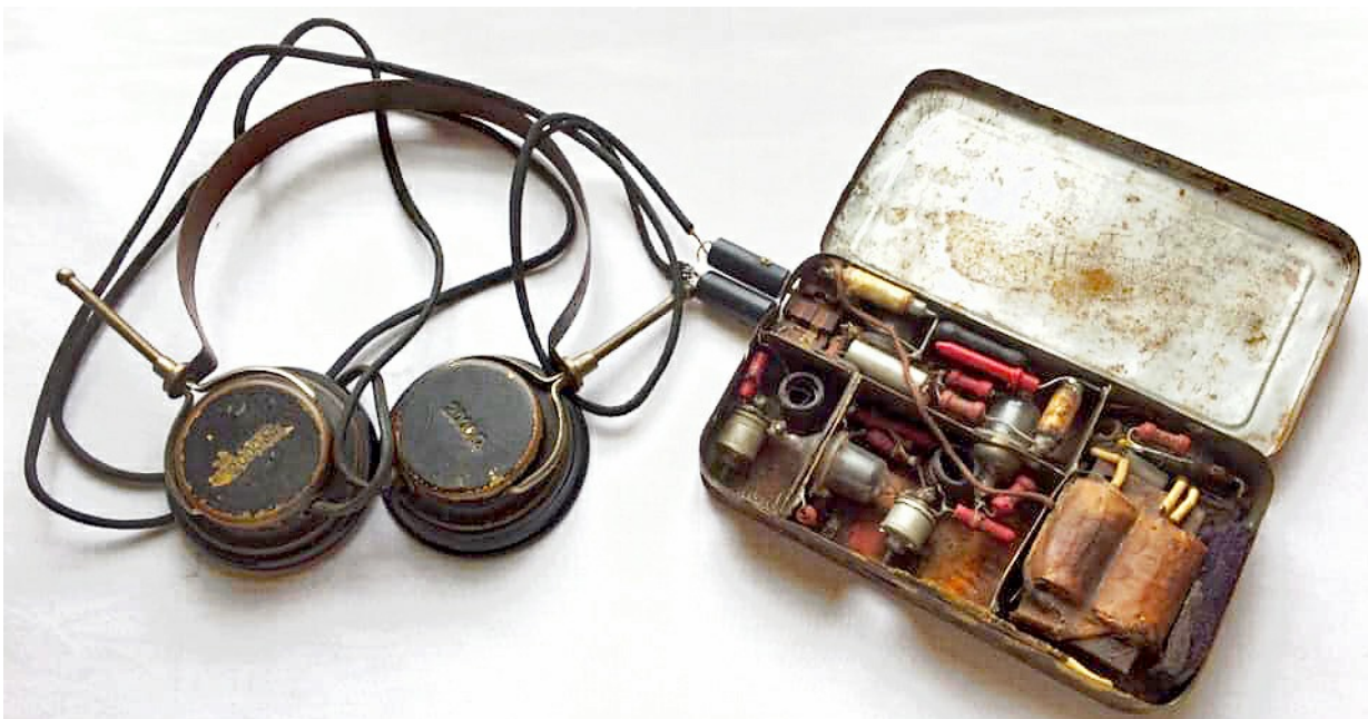
Internal views of an AC mains powered clandestine receiver built in a tobacco tin.
