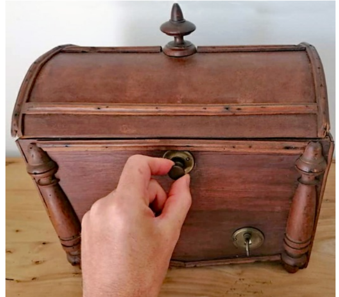
The radio receiver was operated by two keys and a brass knob. The tuning scale and reduction gear were removed.
