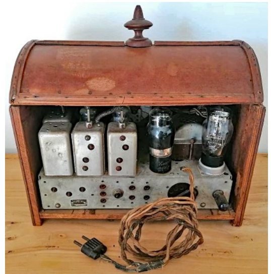
The radio receiver was operated by two keys and a brass knob. The tuning scale and reduction gear were removed.
