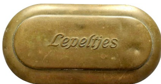
'Teaspoon box' clandestine receiver at about its actual size with reduced size of hinged lid below. ('Lepeltjes' is Dutch for teaspoons).
