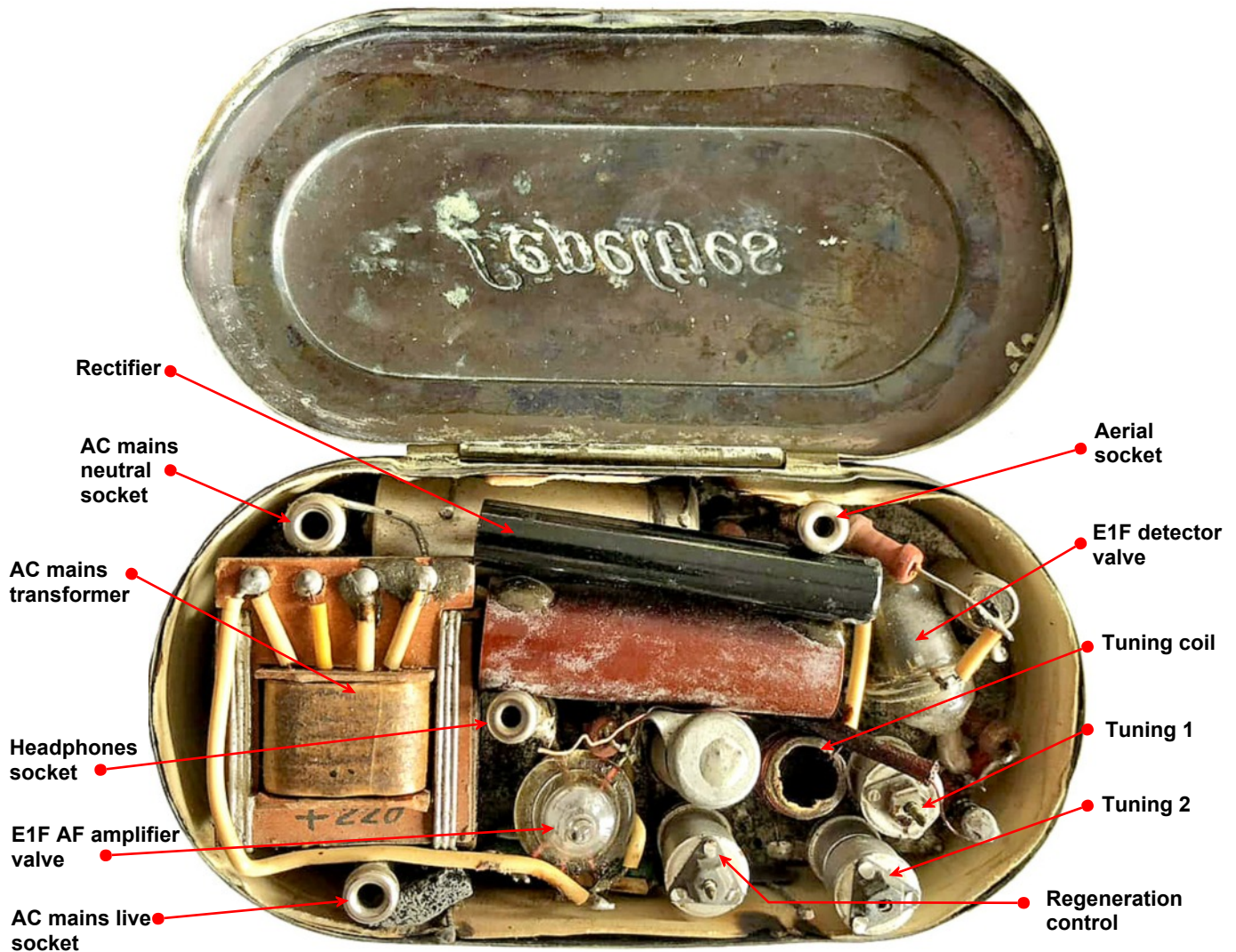
'Teaspoon box' clandestine receiver at about its actual size with reduced size of hinged lid below. ('Lepeltjes' is Dutch for teaspoons).
