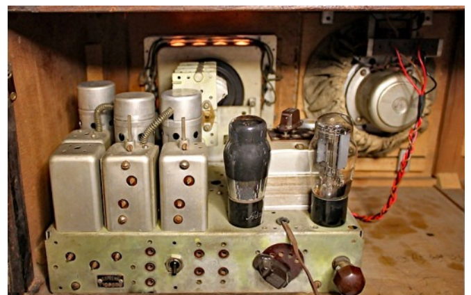
Internal view of the 'Suprema' model 6A, with its back plate detached, showing the chassis with tuning scale and the large loudspeaker.
